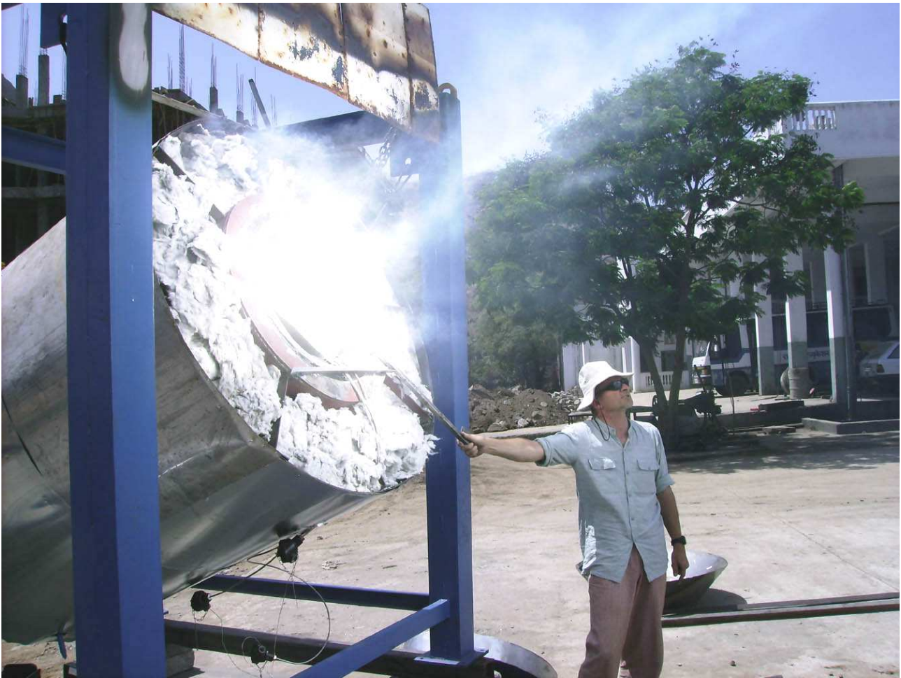
First test of focus size and receiver
