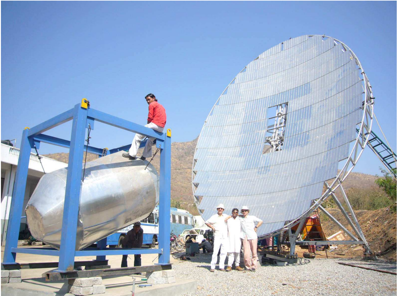
New designed 50m 2 prototype dish and receiver, Shantivan Complex
